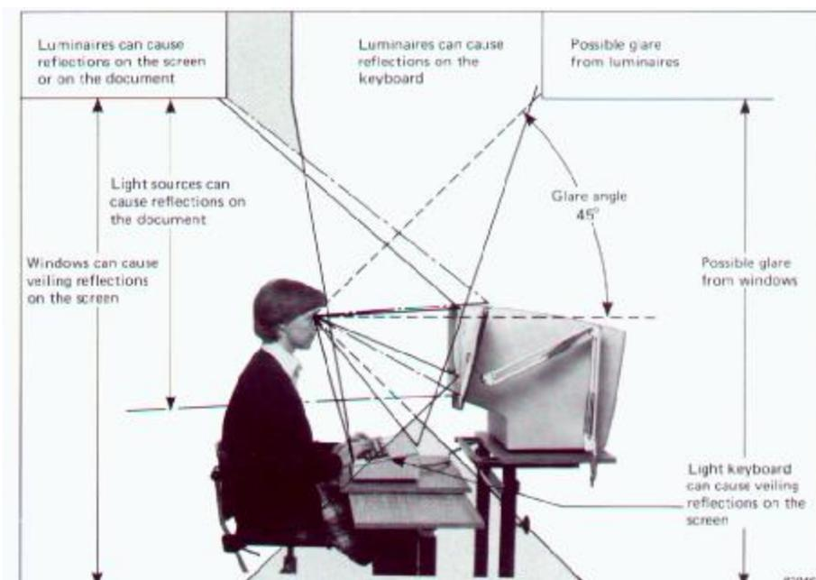
**Fig. 2 The three different task: screen, document and keyboard and zones around the screen terminal where light sources can give reflections or cause glare effects (4)**
