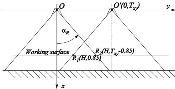
Fig. 2. Position of two luminaires and working surface
