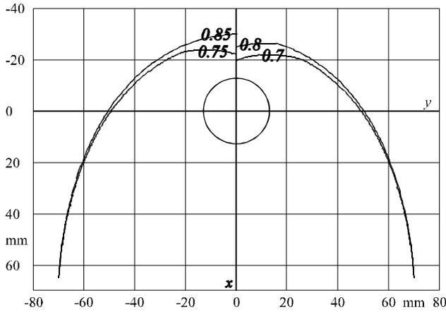
Fig. 5. Reflector profiles giving the assumed illuminance  $E_a$  of the working surface
