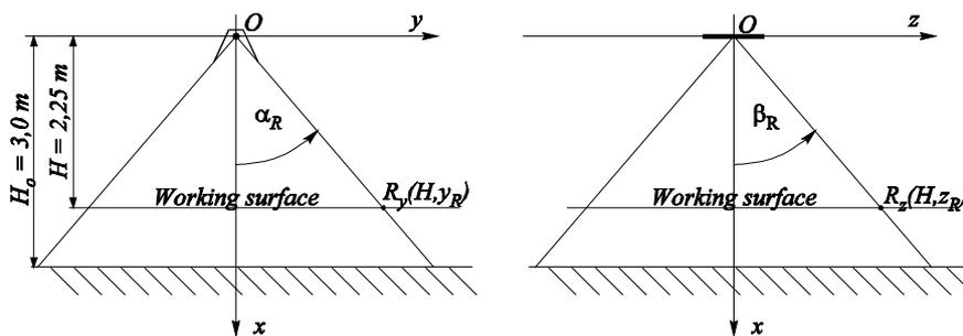
Fig. 1. Position of co-ordinate system, the luminaire and working surface
