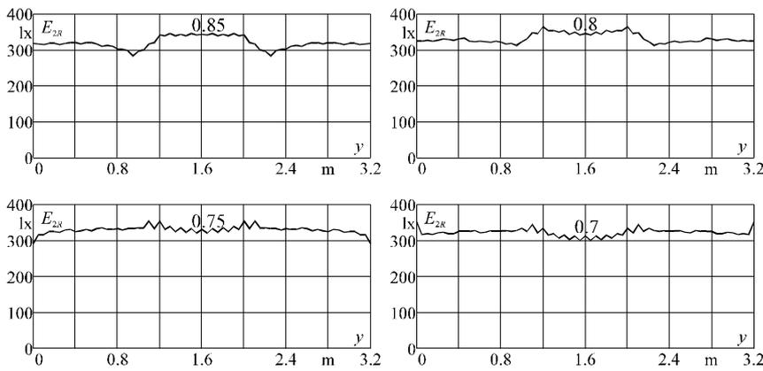
Fig. 6. Illuminance  $E_{2R}$  distribution of the working surface illuminated by the two luminaires 3.2 m apart
