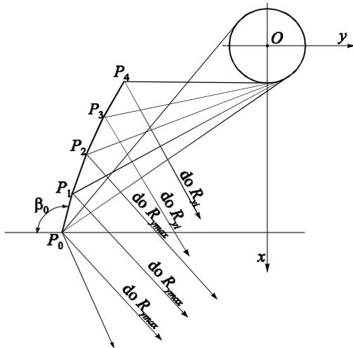
Fig. 4. Diagram of determination of a cylindrical reflector profile by the filling method
