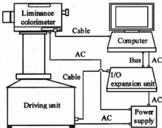
Fig. 1 Block diagram of the measuring instrument
